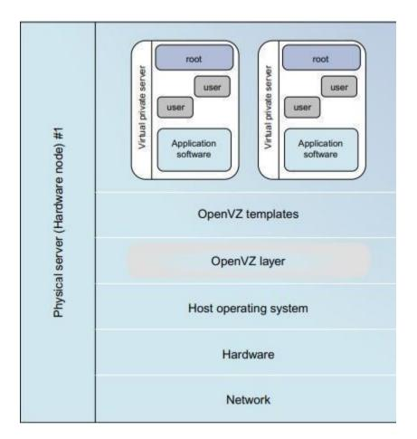
**3 Disadvantages of OS Extensions** The main disadvantage of OS extensions is that all the VMs at operating system level on a single container must have the same kind of guest operating system. That is, although different OS-level VMs may have different operating system distributions, they must pertain to the same operating system family.
