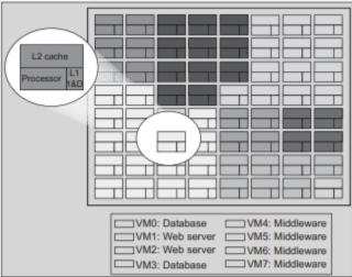
(a) Mapping of VMs into adjacent cores
