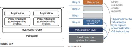
Para-virtualized VM architecture, which involves modifying the guest OS kernel to replace nonvirtualizable instructions with hypercalls for the hypervisor or the VMM to carry out the virtualization process (See Figure 3.8 for more details.)
